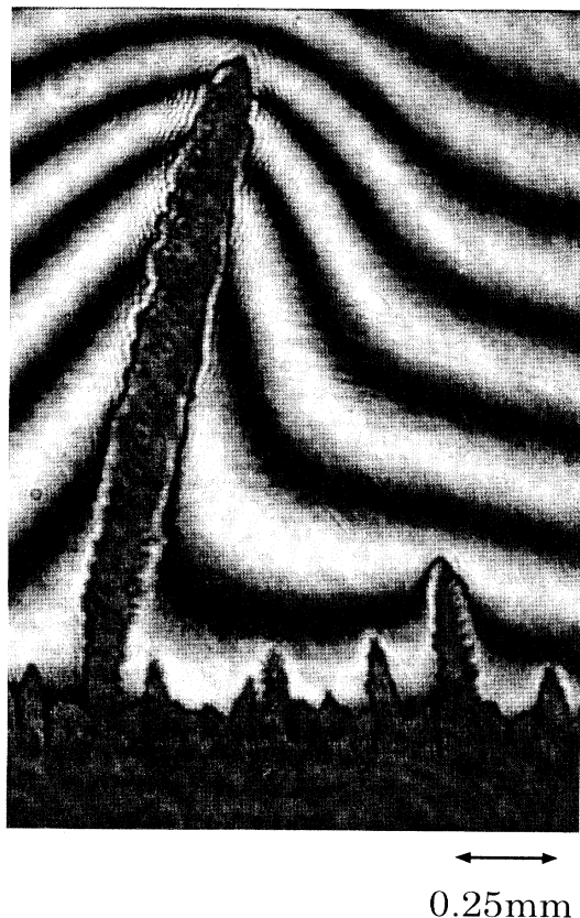
FIG. 12. Microscale interferometric picture of the second destabilization regime (just after the Sand's time) inside the convective roll. The parameter values are [\text{ZnSO}_4] = 1 \text{ mol l}^{-1} , j = 150 \text{ mA cm}^{-2} .
